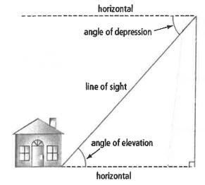
**Ex.** Sean wants to calculate the height of the First Nations Native Totem Pole. He positions his transit 19.0 m to the side of the totem pole and records an angle of elevation of 63° to the top of the totem pole. If the height of Sean's transit is 1.7 m, what is the height of the totem pole, to the nearest tenth of a metre?
